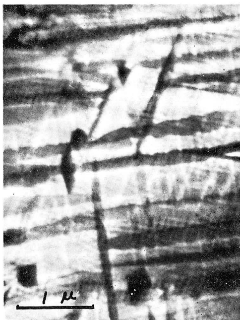
Photo. 49 Al-20% Ag alloy, W.Q., aged for 4 hrs at 200°C. \times 20000
