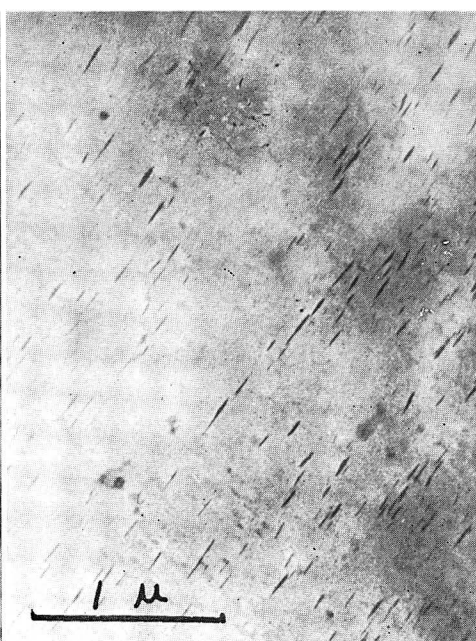
Photo. 34 Al-Cu-Zr alloy, W.Q., 5.0% elong., aged for 1 day at 150°C. \times 25000
