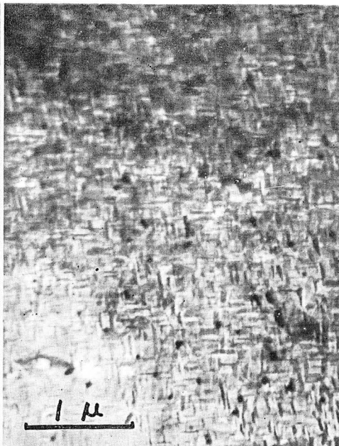
Photo. 52 Al-Ag-Zr alloy, W.Q., 20% rolled, aged for 4 hrs at 200°C. ×20000
