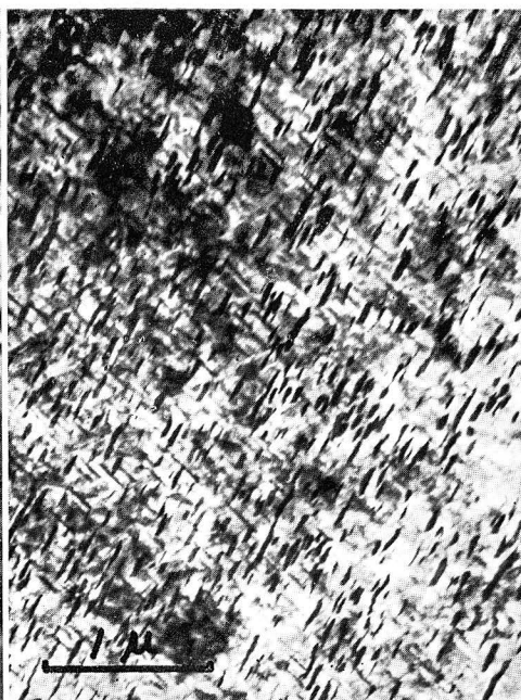
Photo. 50 Al-20% Ag alloy, W.Q., 20% rolled, aged for 4 hrs at 200°C. \times 20000
