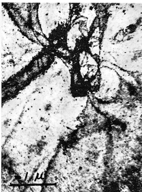
Photo. 44 Al-Ag-Zr alloy, W.Q., aged for 1 day at 110°C. \times 20000
