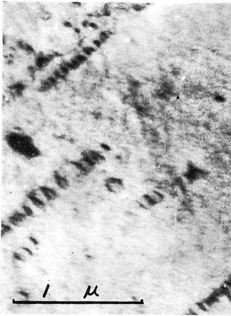
Photo. 19 Al-4% Cu alloy, W.Q., aged for 2 days at 70°C. \times 35000
