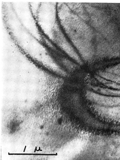
Photo. 33 Al-Cu-Zr alloy, W.Q., aged for 1 day at 150°C. \times 25000
