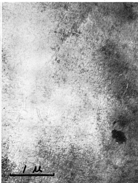
Photo. 46 Al-Ag-Zr alloy, W.Q., aged for 4 days at 110°C. \times 20000
