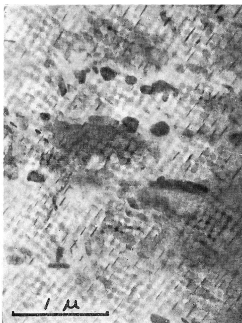
Photo. 29 Al-4% Cu alloy, W.Q., 40% rolled, aged for 1 day at 200°C. ×25000
