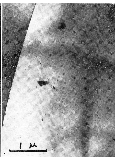
Photo. 42 Al-20% Ag alloy, W.Q., aged for 4 days at 110°C. \times 20000
