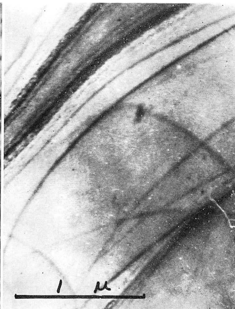
Photo. 24 Al-4% Cu alloy, W.Q., 5.0% elong., aged for 4 days at 110°C. \times 35000
