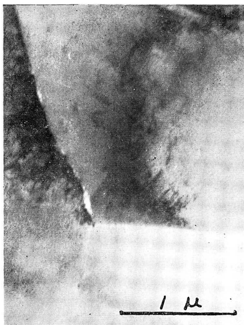
Photo. 31 Al-Cu-Zr alloy, W.Q., aged for 70 days at 70°C. \times 30000
