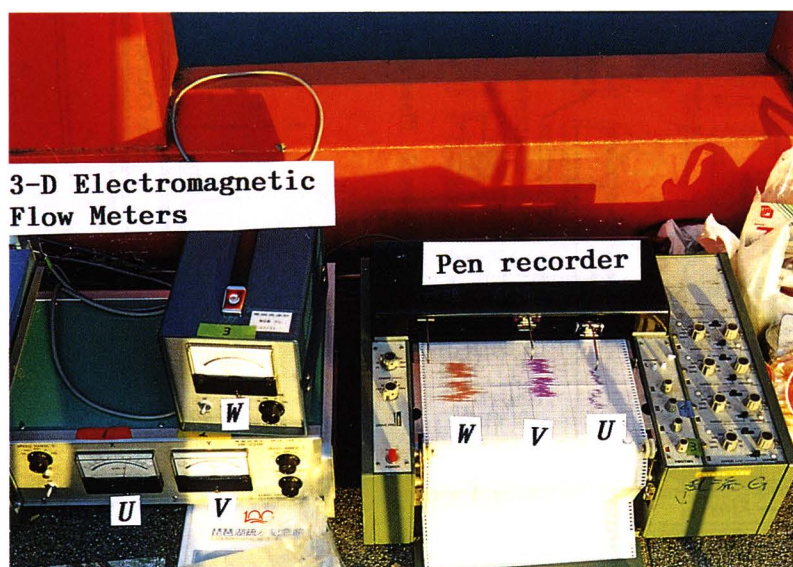
Figure 4 Photograph of measurement system.
