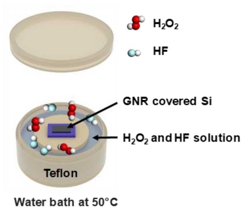
Figure 4.2. Illustration of the Si vapor-etching process. The etchant solution consisted of 25 mL of 46% HF and 0.5 mL of 30% H 2 O 2 . Etching proceeded at 50°C for 1 h.
