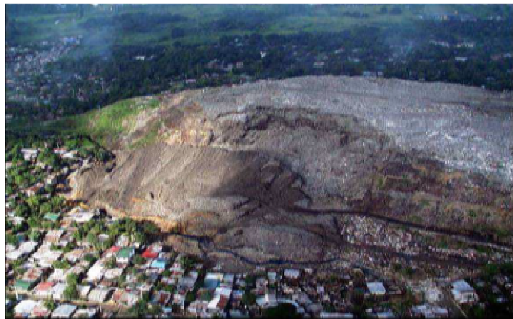
Fig. 2.5 Aerial view of Payatas landfill failure in Philippine (Zekkos 2005).
