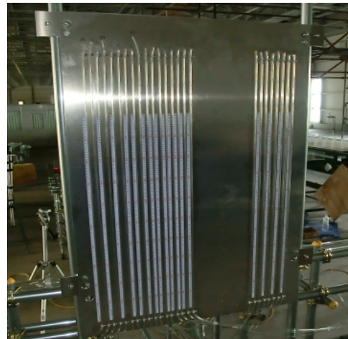
Figure 3.10 Panel of piezometric tubes
