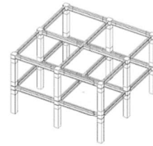
Fig.5 Mesh of a frame made by assembling component meshes
