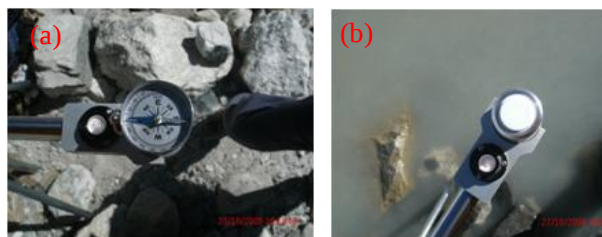
Photo 3 Albedo measurements of (a) Debris at the Imja glacier, (b) The glacial lake water
