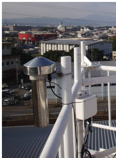
Photo 3 Hygrometer with hygroscopic sensor (in the shelter for ventilation)
