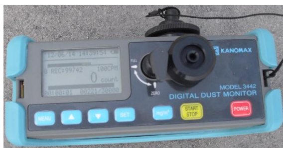
Photo 2 Digital dust meter
