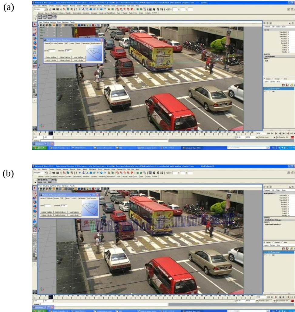
Fig. 3.7 (a) The track of pedestrian route is selected, (b) After select the route of pedestrian, the button Output Cylinder is click to obtain the coordinate x- and y- axis in each 0.5 second
