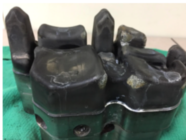
1. Die condition before repair
