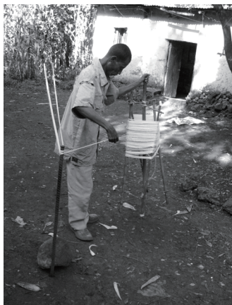
Fig. 12. A Man in Bahir Dar is warping thread with two sticks ( Denker, Chahel ) and one stick ( Ainet ).
