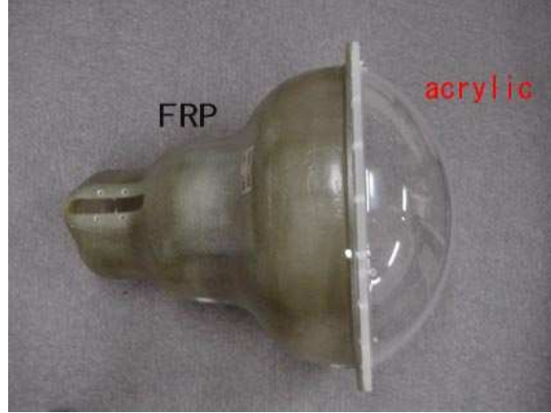
FIGURE 2.6: PMT case for 20-inch ID PMT since SK-II period.
