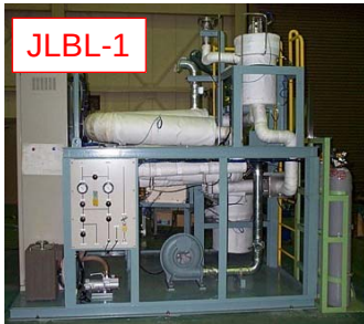
JLBL (JAEA Lead-Bismuth flow Loop)
