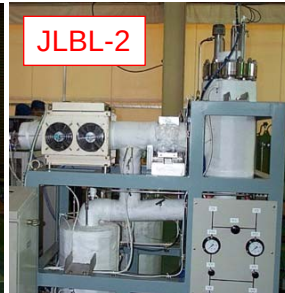
JLBL (JAEA Lead-Bismuth flow Loop)
