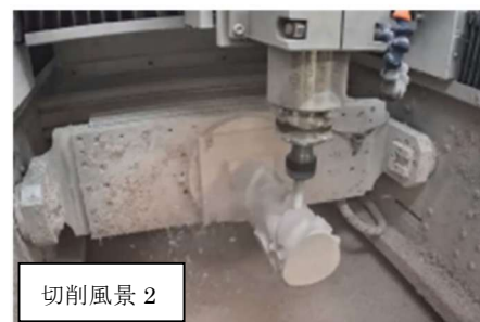
Fig.15 Performance Verification Test 2–Machining of a three-dimensional shape with rotary axis.
