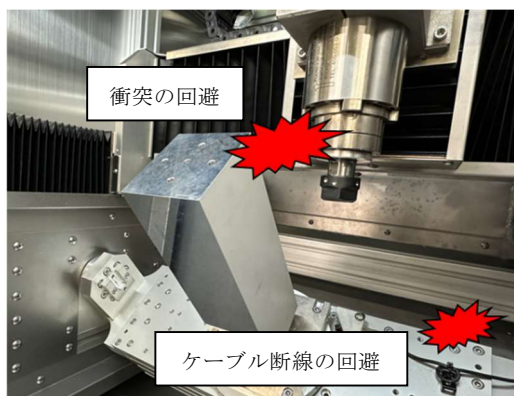
Fig.6 Examples of collision and cable disconnection risks due to insufficient CAD/CAM planning.
