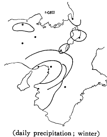
Fig. 3.2 Isolines of the inter-station correlation coefficients.
