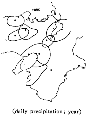
Fig. 3.1 Isolines of the inter-station correlation coefficients.
