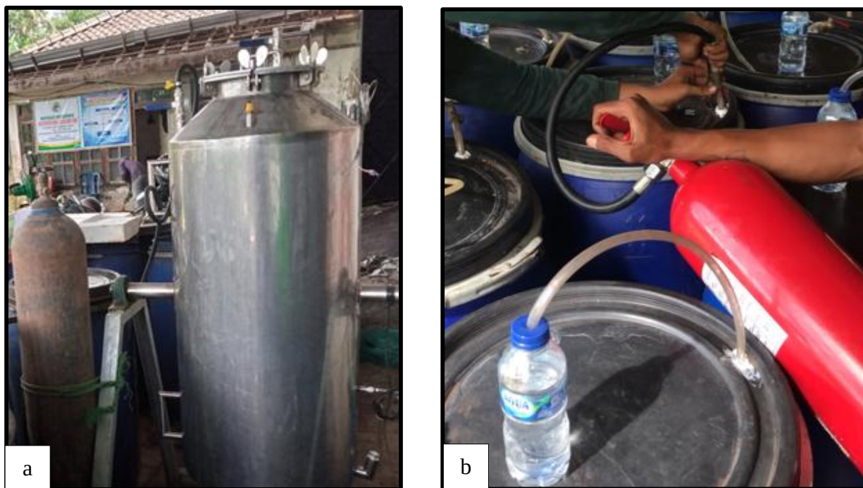
Figure 2.9 (a) Stainless reactor with injection of CO 2 , (b) Plastic reactor injection of CO 2 at lower pressure
