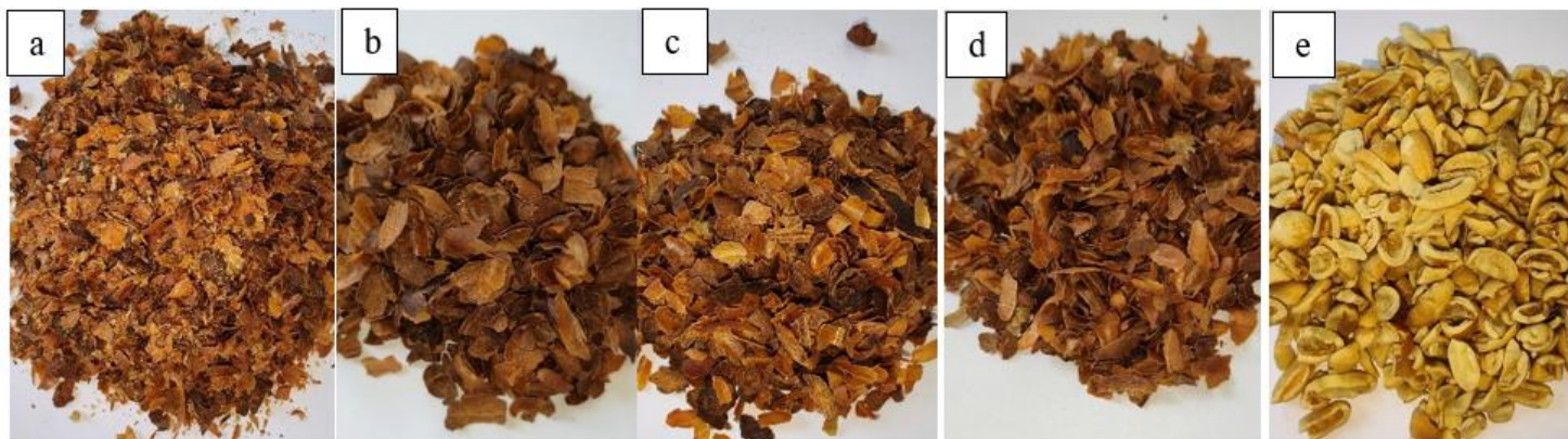
Figure 7.13 Raw HS (a) ; Sorted HS of size 7.5mm (b), 6.5mm (c), 5.5mm (d), and pixel (e)
