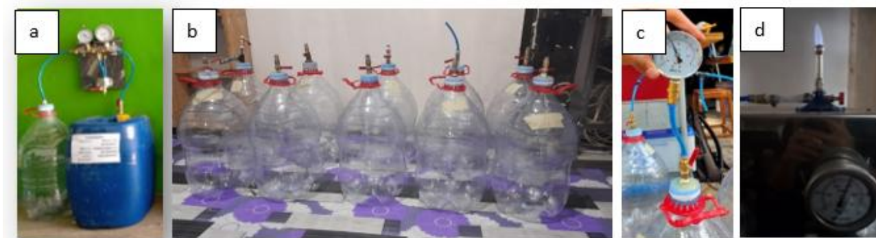
Figure 5.3 (a) Small 20L reactor, (b) 15L gas storage containers, (c) gas pressure gauge on storage, (d) biogas burning
