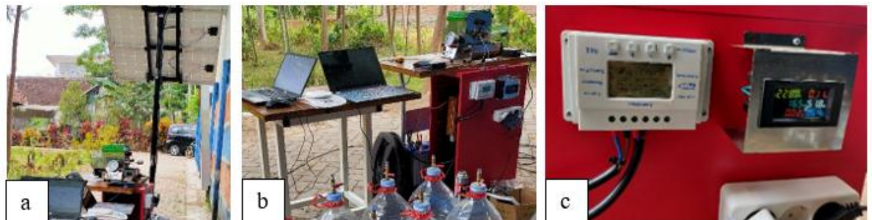
Figure 7.3 (a) Solar panel, (b) Coffee roaster machine, (c) AC power meter (black), DC power meter (white)
