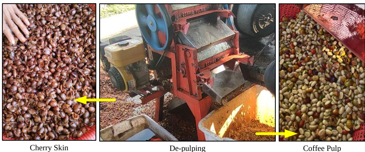
Figure 2.3 De-pulping process for separation cherry skin and coffee pulp
