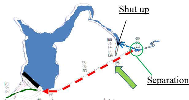
Fig. 5: Nunobiki Reservoir Bypass Tunnel
