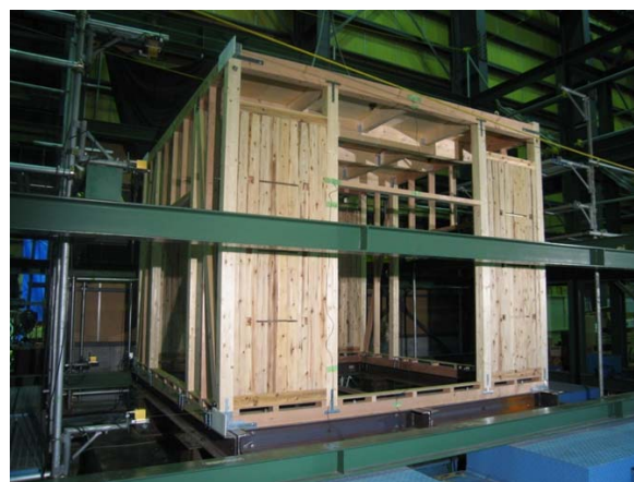
Photo 3 A specimen for a shaking table test of a one-room wooden house model with “Wall-of-Columns” reinforcements.
