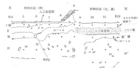
Fig.5 Figure of the log of the wall in trench restored before the fault movement. The left side is the figure of south half in west wall and the right side is the one of north half in east wall (seen from reverse direction). And the layer of silt is put on the layer III' of north half temporally.
