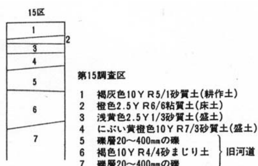
Fig.4 Columnar section of soils in the 15 th division from the archeological report. The layers No.1~4 were researched in the archeological excavation and the layers No.5~7 correspond to those in the trench excavation.
