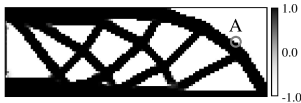
Fig. 8 Distribution of the design variable \phi using the proposed MPPM
