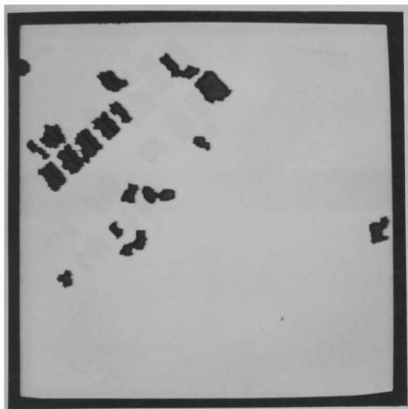
Fig. 6.14 Houses recognized by the HOUSE 2 subsystem using the multispectral properties of the already recognized houses.
