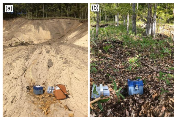
Photo 16 Microtremour observation on the sliding surface (a) and on the neighboring slope (b) in Tomisato area
