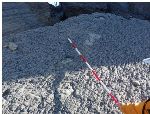
Photo 12 Surface of the outcropped bedrock on the source area of Hidaka-Horonai landslide
