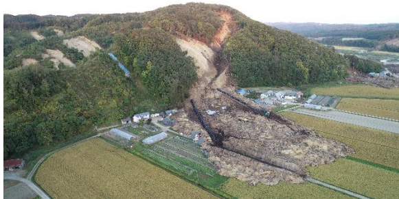
Photo 8 A fluidized landslide on west side of the slope shown in Photo 6 (Taken on September 28, 2018)
