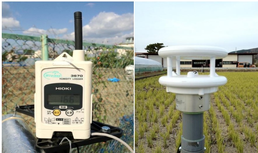
Figure 5.6. Thermometer and anemometer for monitoring temperature and wind.
