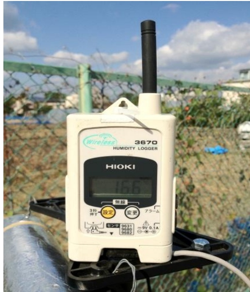
Figure 2.10. Thermometer for monitoring surrounding temperature to adjust the sound speed.
