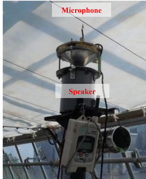
Figure 5.3. Modified transmitter/receiver used for self-calibration.
