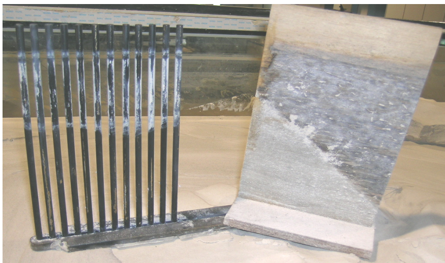
Photo 2.1 Permeable (Left) and Impermeable (Right) Spur Dykes Used in the Experiments
