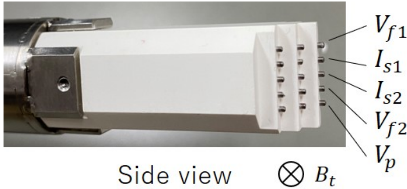
Figure 5.4: Side view of the probe head and its channel setup.
