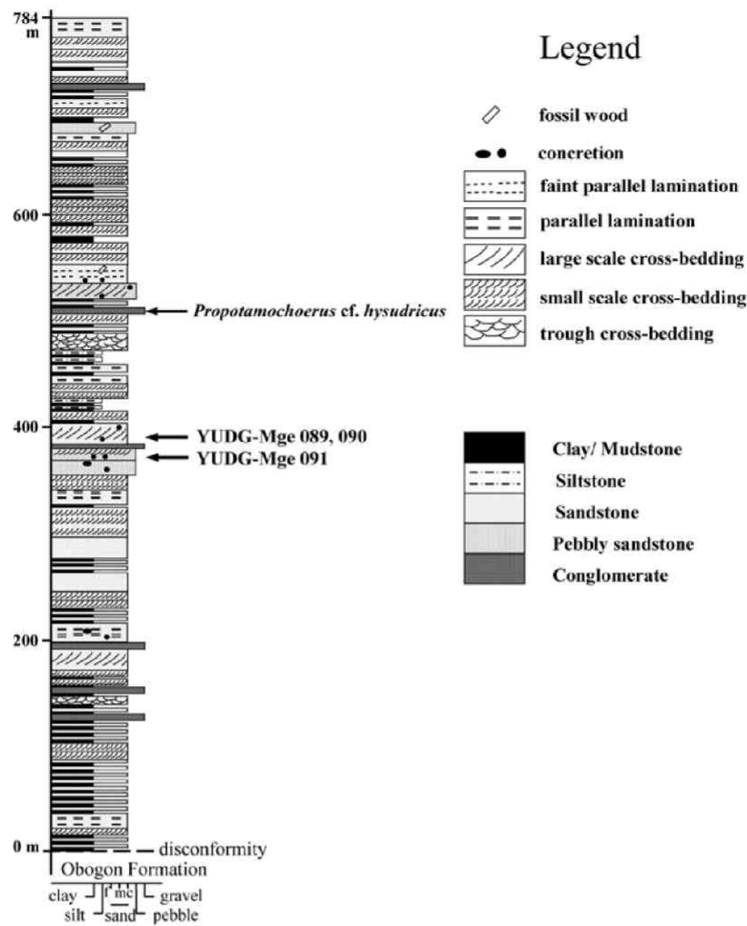
Figure 2. Columnar section of the lower part of the Irrawaddy Formation at the fossil locality Tebingan (95° 08'15.2"E; 19°57'7.6"N) in the west of Tebingan Village, Migyaungye area, with indication of the strata which yielded suid fossils. Abbreviations: f, fine-grained; m, medium-grained; c, coarse-grained.
