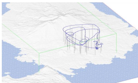
Fig. 4 Flight locus of UAV in Sakurajima by GPS, 24 February 2012
