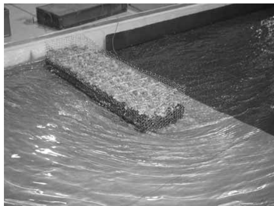
Photo 6 Laboratory experiment on rubble mound groin (Case-A, i.e. h < h_g ).
