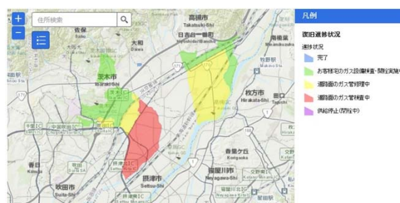
Fig. 26 Progress of recovery of natural gas pipelines as of June 21 st 2018 (Osaka Gas, 2018c)
