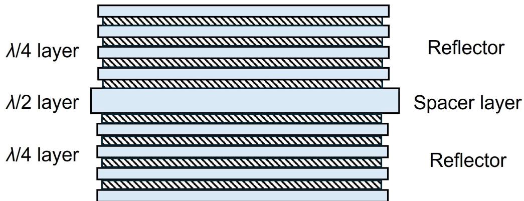
Figure 3.1. The structure of a Fabry–Pérot filter structure.
