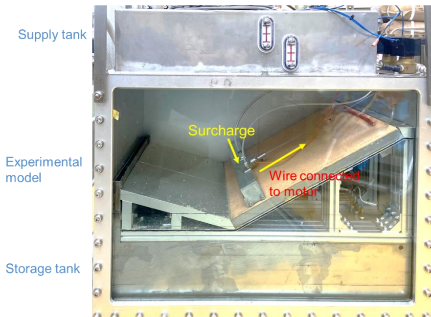
Figure 3-11 Front of centrifuge model container
