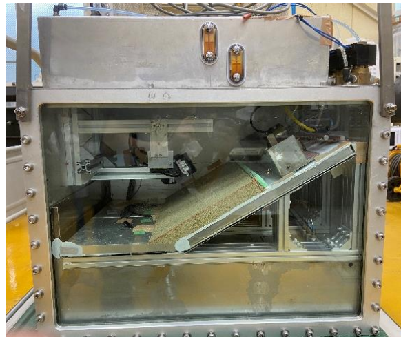
Figure 5-12 Installation of supply top tank
