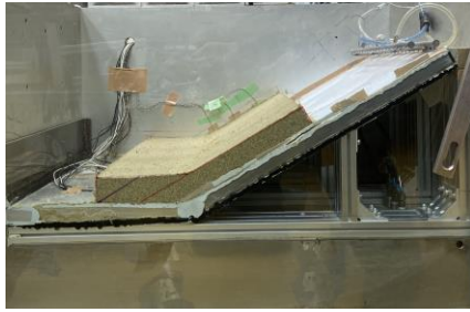
(a) Compaction and cutting berm near toe
