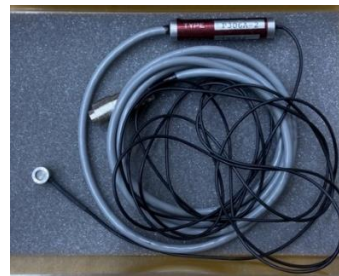
b) Cable of pore water pressure transducer
