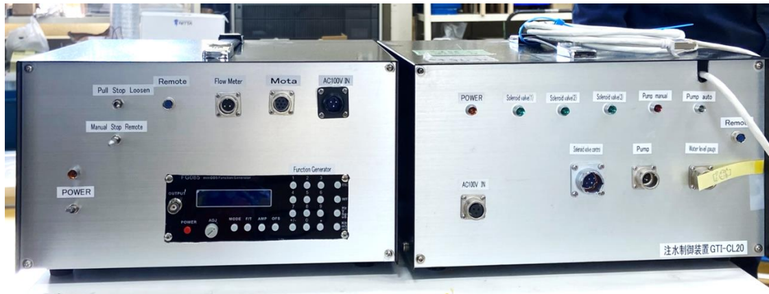
Figure 3-17 Control boxes of water supplementation and surcharge controller.
