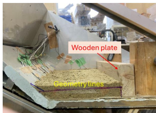
Figure 6-8 Rotation of soil chamber and compaction
