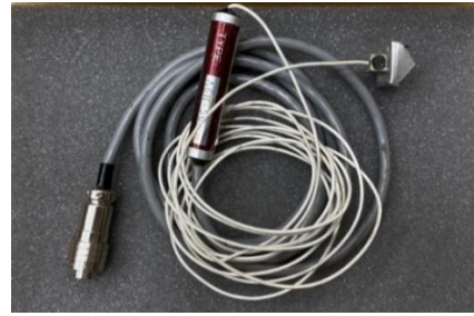
b) Cable of Accelerometer
