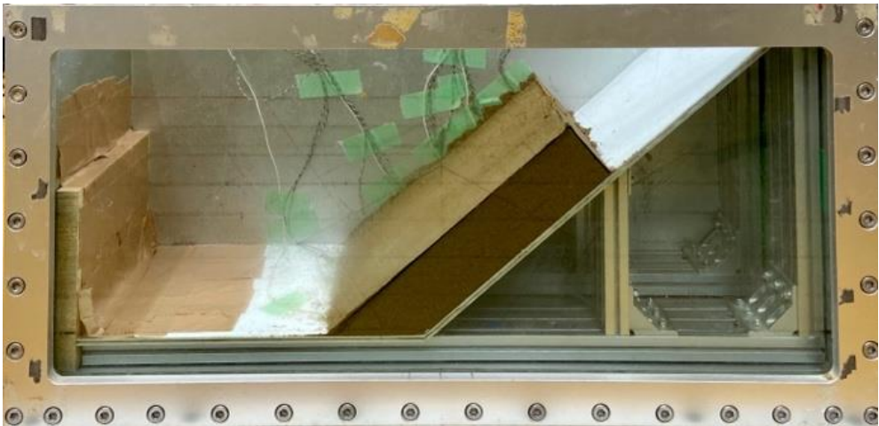
Figure 8-5 Soil chamber and model (model scale)
