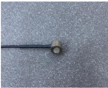
a) Pore water pressure transducer
