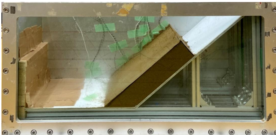
Figure 3-25 Centrifugal model for dynamic experiment
