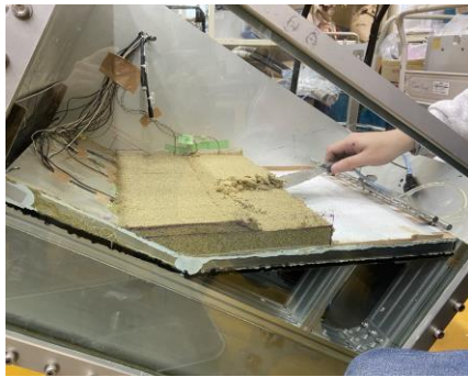
(a) Compaction and cutting berm near toe
