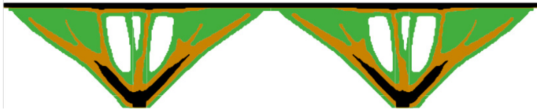
FIGURE 4.19: Optimized 2D three-material bridge without the outer coating using the ordered SIMP method.
