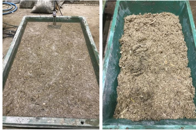
Figure 3.2 Washing (left) and drying (right) process of the bagasse fiber
