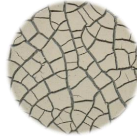
Fig. 1 Desiccation cracking pattern of soil.
