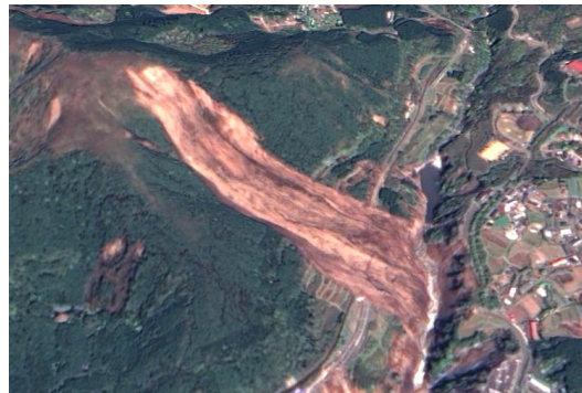
Fig. 2 Three-dimensional ZY3 oblique-image (2m resolution) of Aso Bridge landslide (32.886, 130.983). View to north, shoted on April 20, 2016
