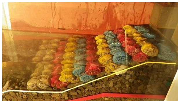
Photo 7 Experiment for stability of net-unit in waves
