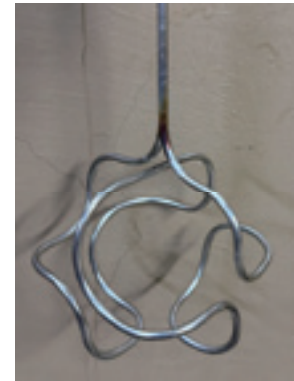
Fig.3 Outlook of the water-cooling hollow cathode made of 3.2 mm-O.D. SUS316L tube
