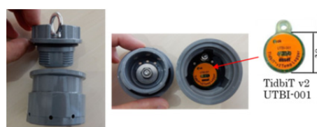
Fig. 2 Water temperature data logger and its small housing.
