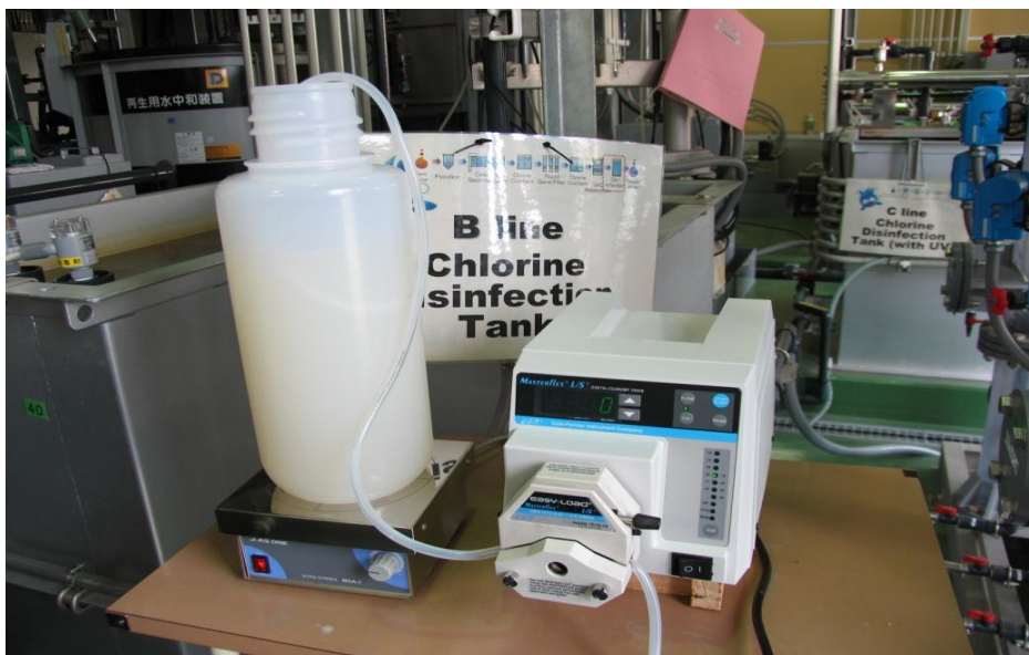
Figure 5-5 E.coli spiking solution and pump (Cultured E. coli was suspended in 5L of test water)
