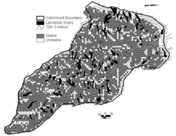
Fig. 6 Landslide scars and Stability map of area by steady state model
