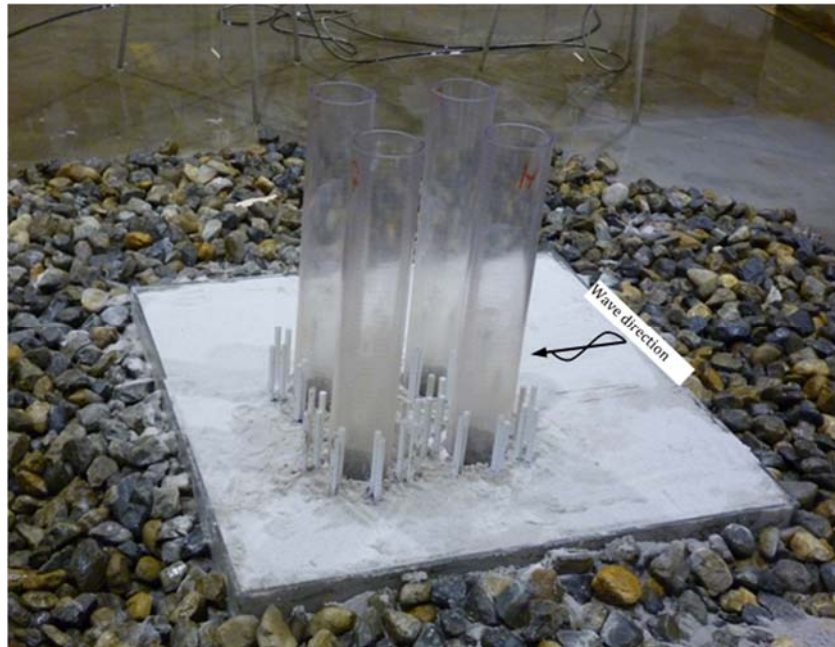
Figure 2-23. Photo of the four piles experimental model
