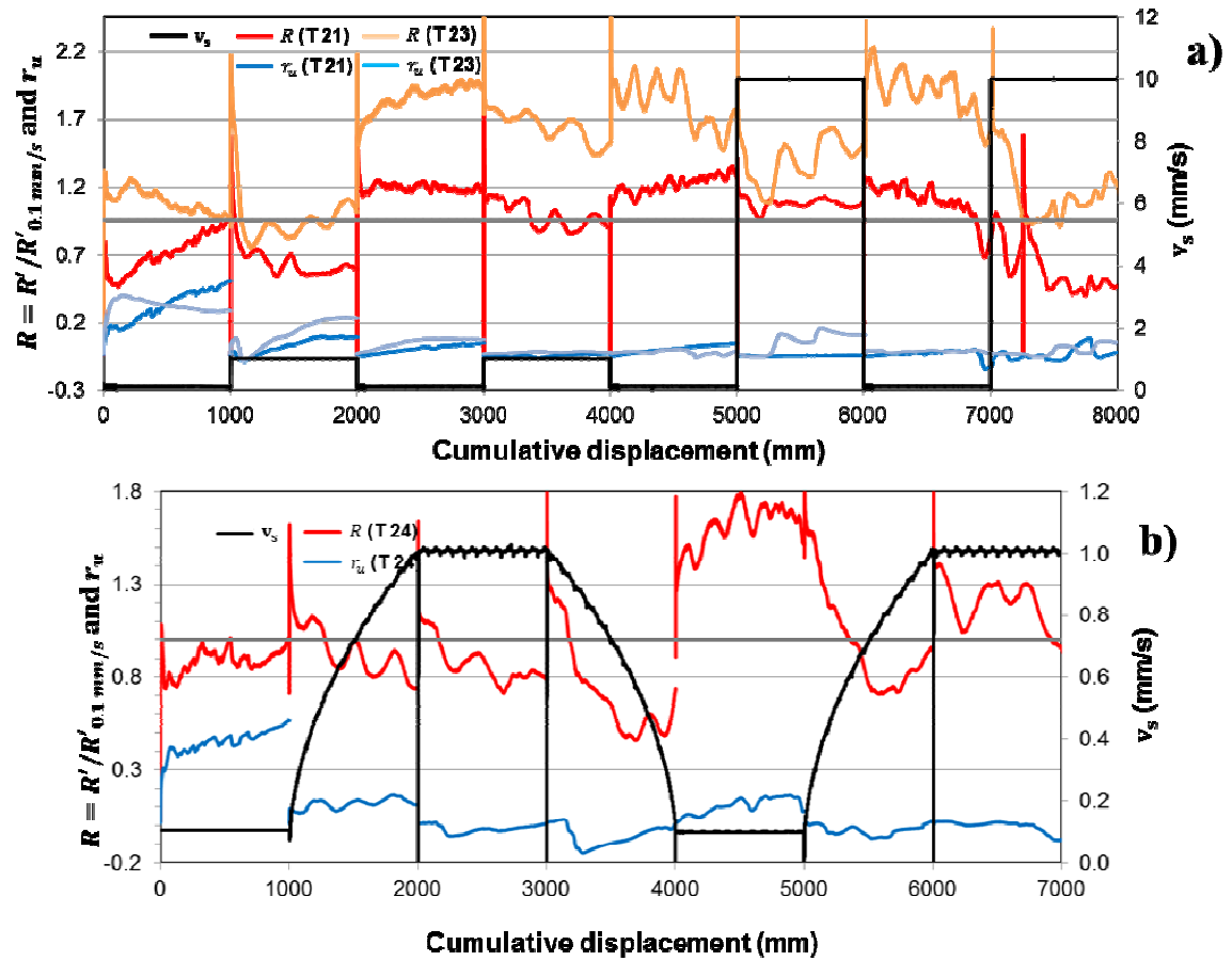
Figure 4.13 Cumulative displacement and friction coefficient and pore pressure ratio of multi-stage tests conducted on SB 30 specimens a) T 21 and T 23 (8 stages) and b) T 24 (7 stages).
