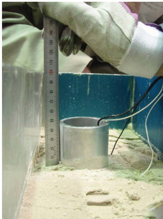
Fig. 2.8 Uplifted manhole after shaking (CS2).
