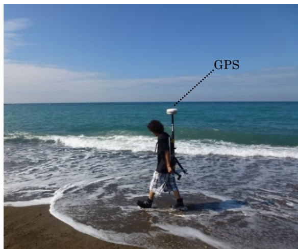
Photo 2 Walking terrain measurement on land/extremely shallow regions using RTK-GPS survey system.
