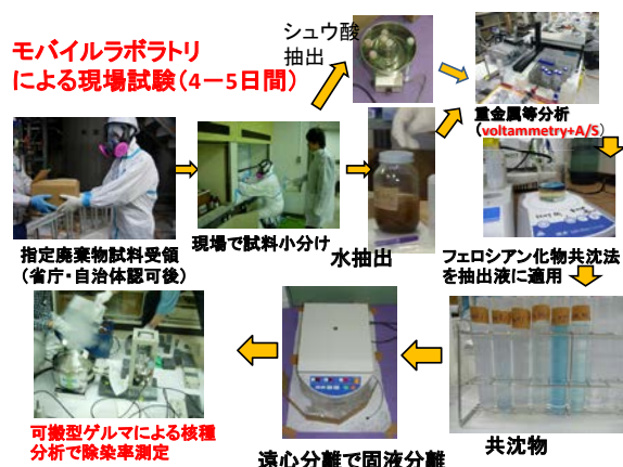
Fig. 1 Procedures of on-site test treating designated waste samples containing radioactive cesium
