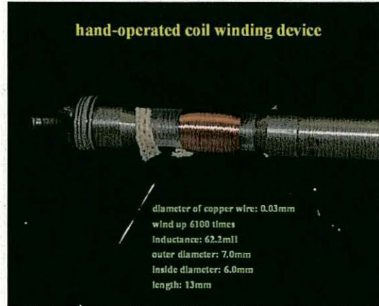
Fig.1: Hand-operated coil, 0.03mm copper 6100 times
