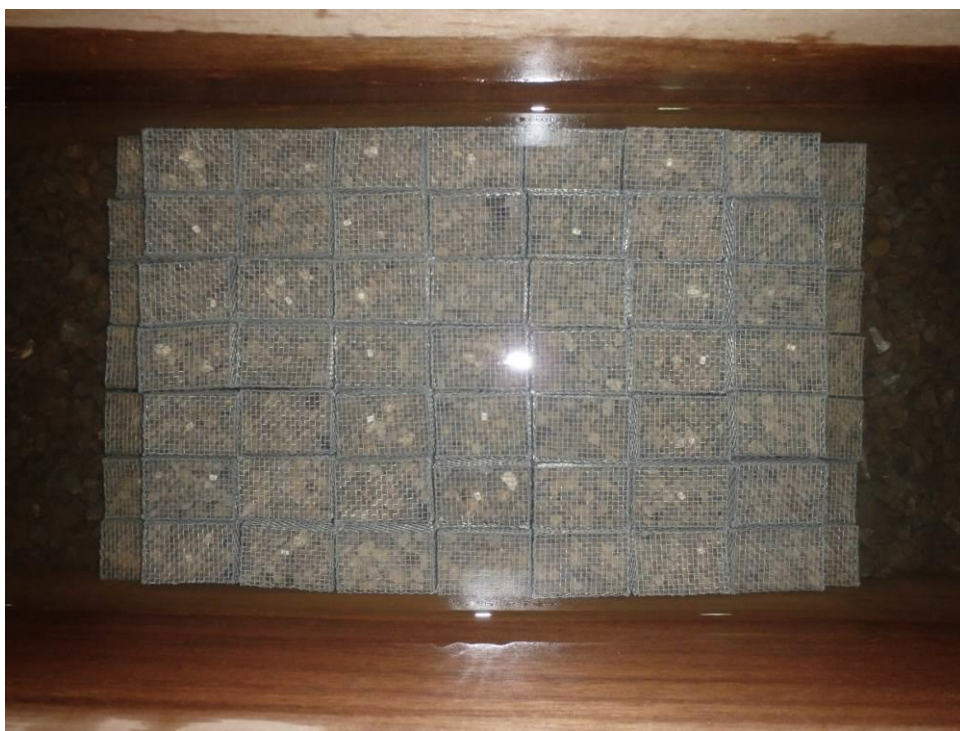
Photo 3A Effect by tsunami action ( no damage, tsunami height=13.7cm, water depth=20cm)
