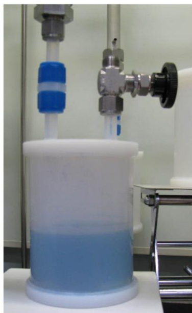
Fig. S1 Photographs of PFA reactors for (a) Reactor A or C and (b) Reactor B in Fig. 2. The reactor in the photograph (b) contains ~500 mL of HF with \text{AgFAsF}_6 .
