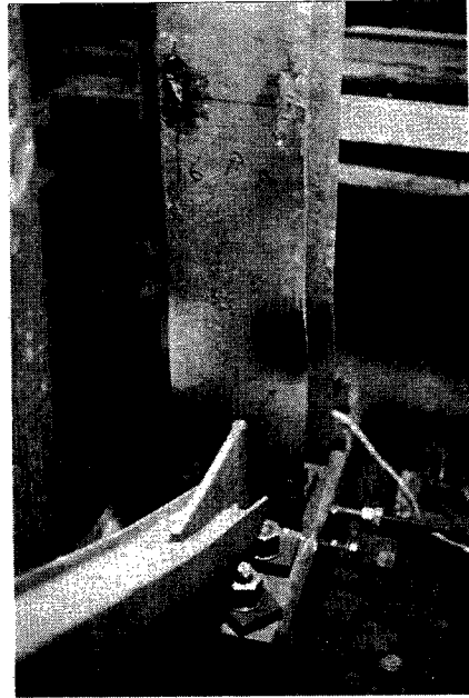
Photo. 9 Local buckling of column bottom (BC5).
