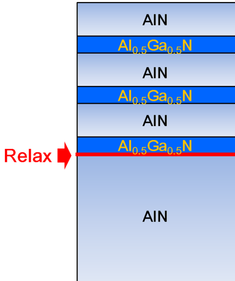
Figure 4.27: Schematic images of (a) \text{Al}_{0.5}\text{Ga}_{0.5}\text{N}/\text{AlN} 3QW and (b) \text{Al}_{0.55}\text{Ga}_{0.45}\text{N}/\text{Al}_{0.75}\text{Ga}_{0.25}\text{N} 3QW, which has a 50-nm-thick \text{Al}_{0.75}\text{Ga}_{0.25}\text{N} relax layer to suppress nonradiative recombinations in the well layers due to MDs. For both of the QWs, the well and barrier layer thicknesses are about 1.5 and 15 nm, respectively.
